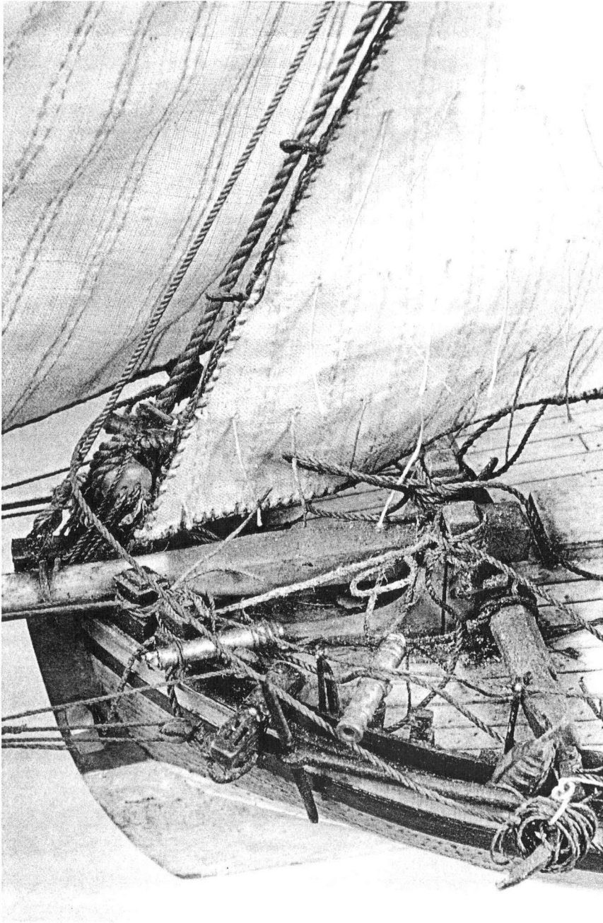
10. Detail of the forestay with its deadeye and lanyard, preventer stay and the square heel of the bowsprit. The windlass on this particular model is unconventional for, having no carrick bits, the spindle ends are supported directly on the bulwarks. (NMM)
