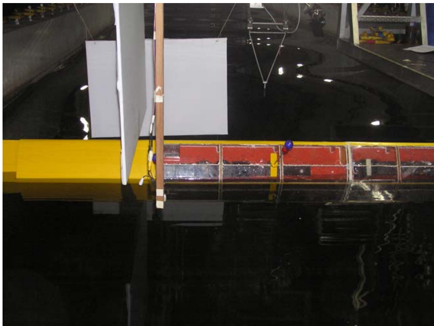
Figure F.9 Image processing on damage stability experiment - condition 3
