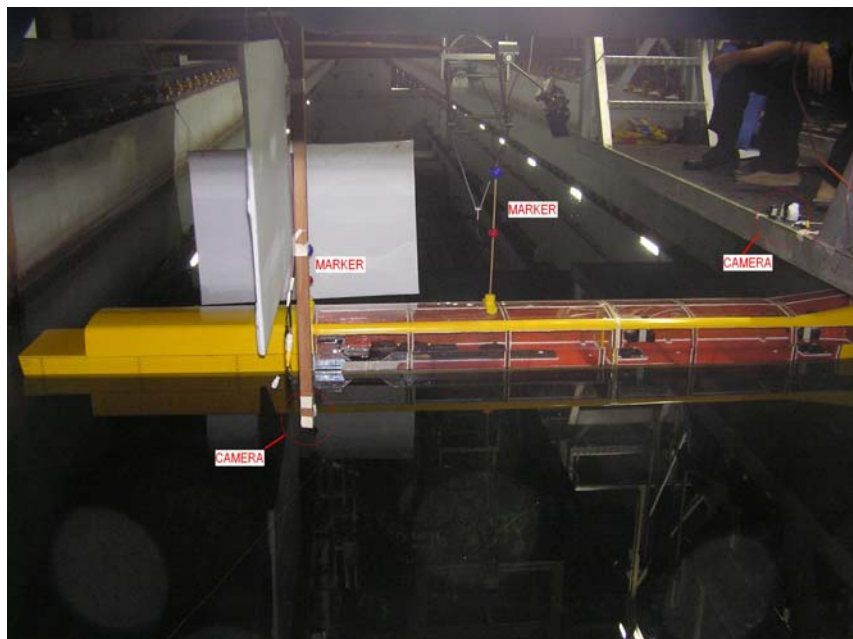
Figure F.5 Cameras and markers set-up
