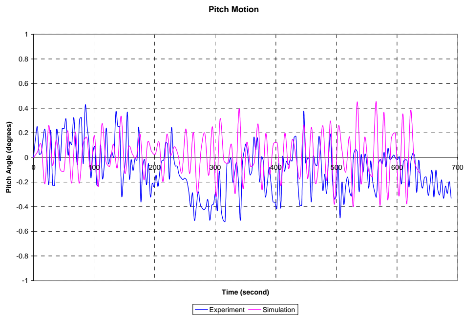
Figure 7.3: Pitch motion (case A): Comparison of experiment and simulation
