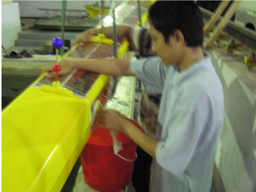
Figure F.4 Measure the weight of water ingress for each time step
