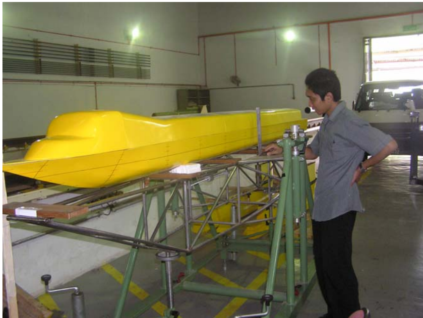
Figure F.1 Ship model on swinging frame
