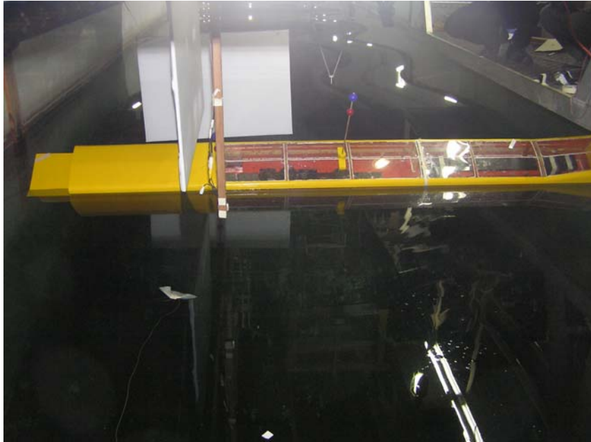
Figure F.8 Image processing on damage stability experiment - condition 2
