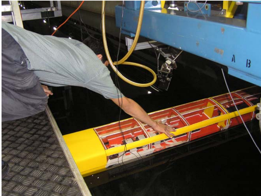
Figure F.2 Roll decay test
