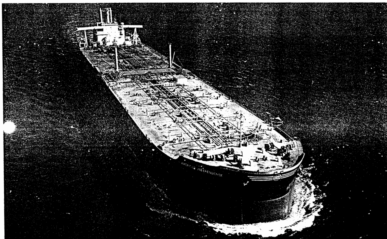
Fig. 7 SS AMERICAN INDEPENDENCE—Very large crude carrier built at the Bethlehem Steel Corporation, Sparrows Point Shipyard in 1977 for Gulf Trading and Transportation Company; Molded dimensions 335.3 m (1,100 ft) by 54.3 m (178 ft) by 26.2 m (86 ft)
