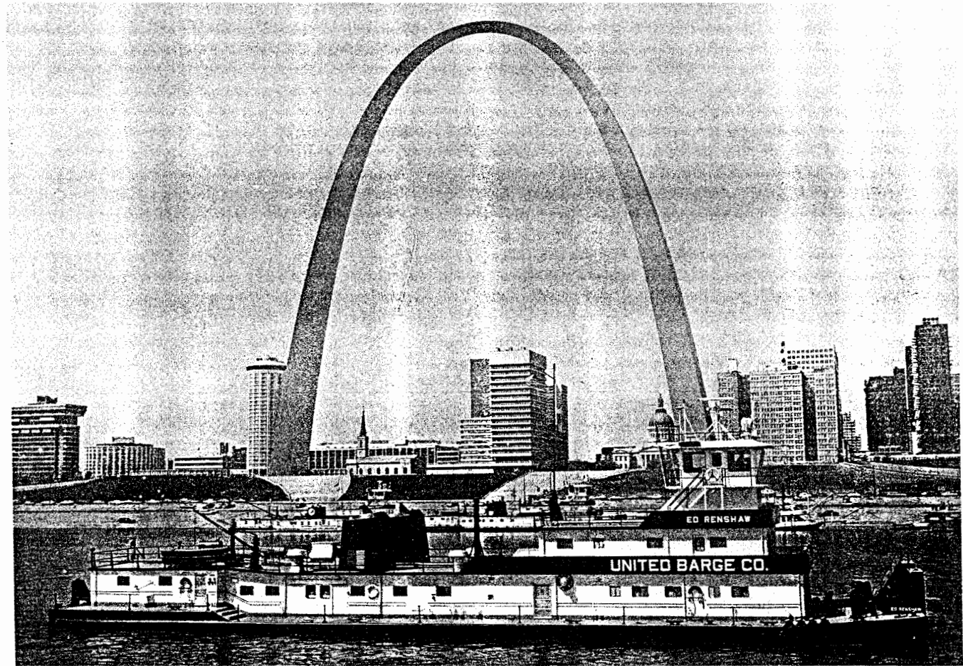
Fig. 13 M/V ED RENSHAW—Western River tow boat built in 1977 by St. Louis Ship for United Barge Company; Molded dimensions 51.8 m (170 ft) by 13.7 m (45 ft) by 3.4 m (11 ft)
