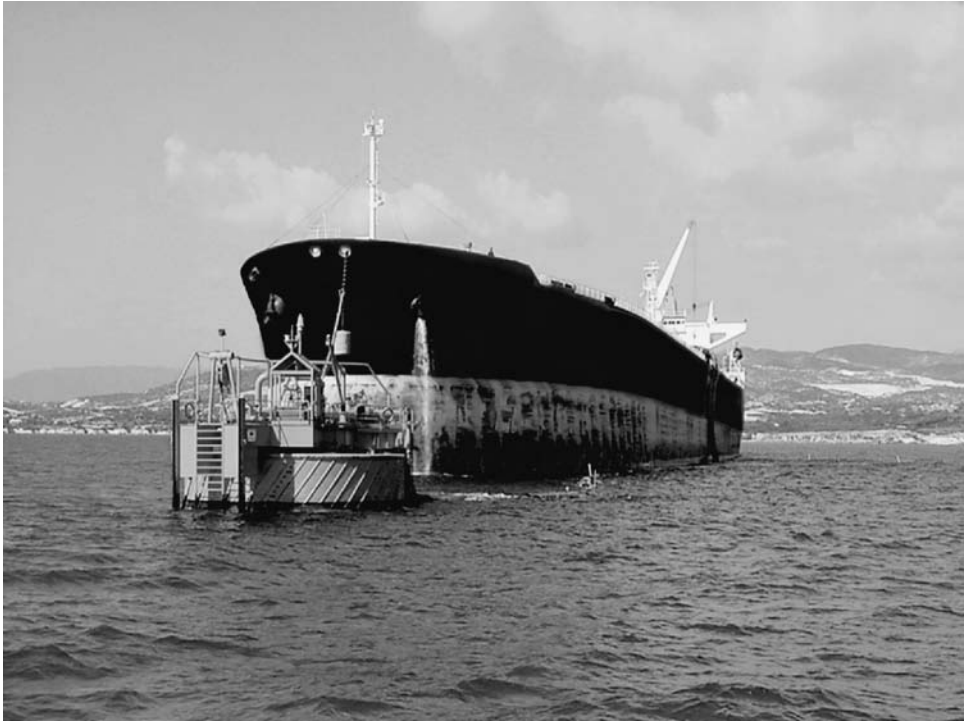
Figure 9.11. ( cont. ) (c) A photograph of a CALM arrangement with an FPSO (courtesy of SBM Offshore NV).
