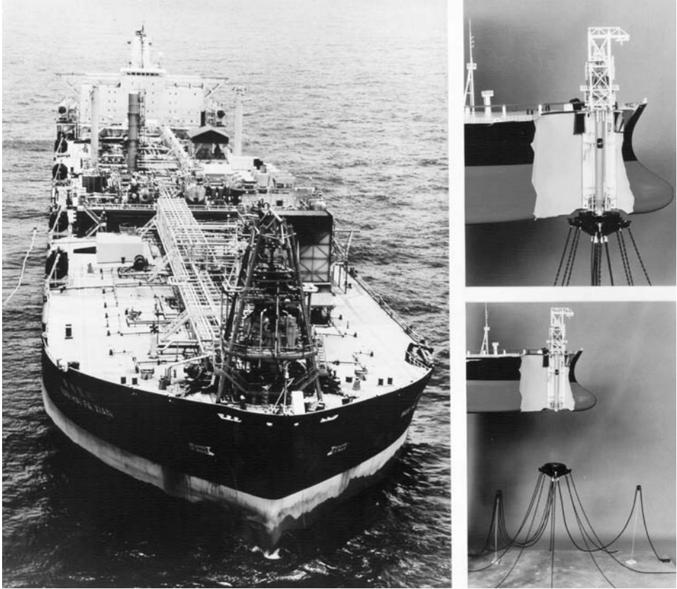
Figure 9.17. (a) An FPSO with an internal disconnectable turret-mooring system and its schematic (courtesy of SBM Offshore NV).
