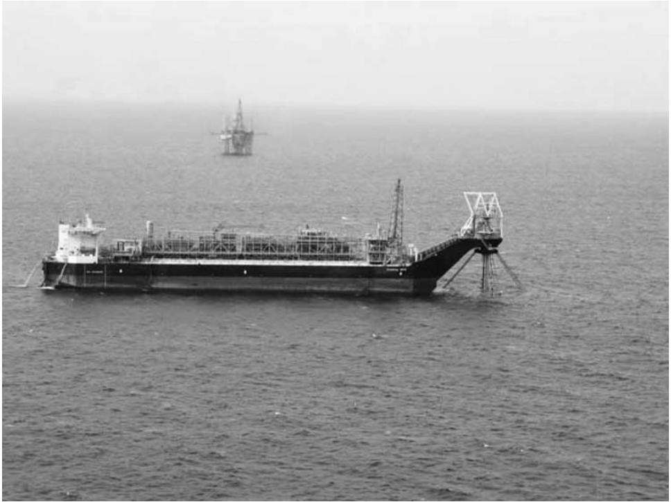
Figure 9.16. An FPSO with an external turret-mooring system (courtesy of Samsung Heavy Industries).
