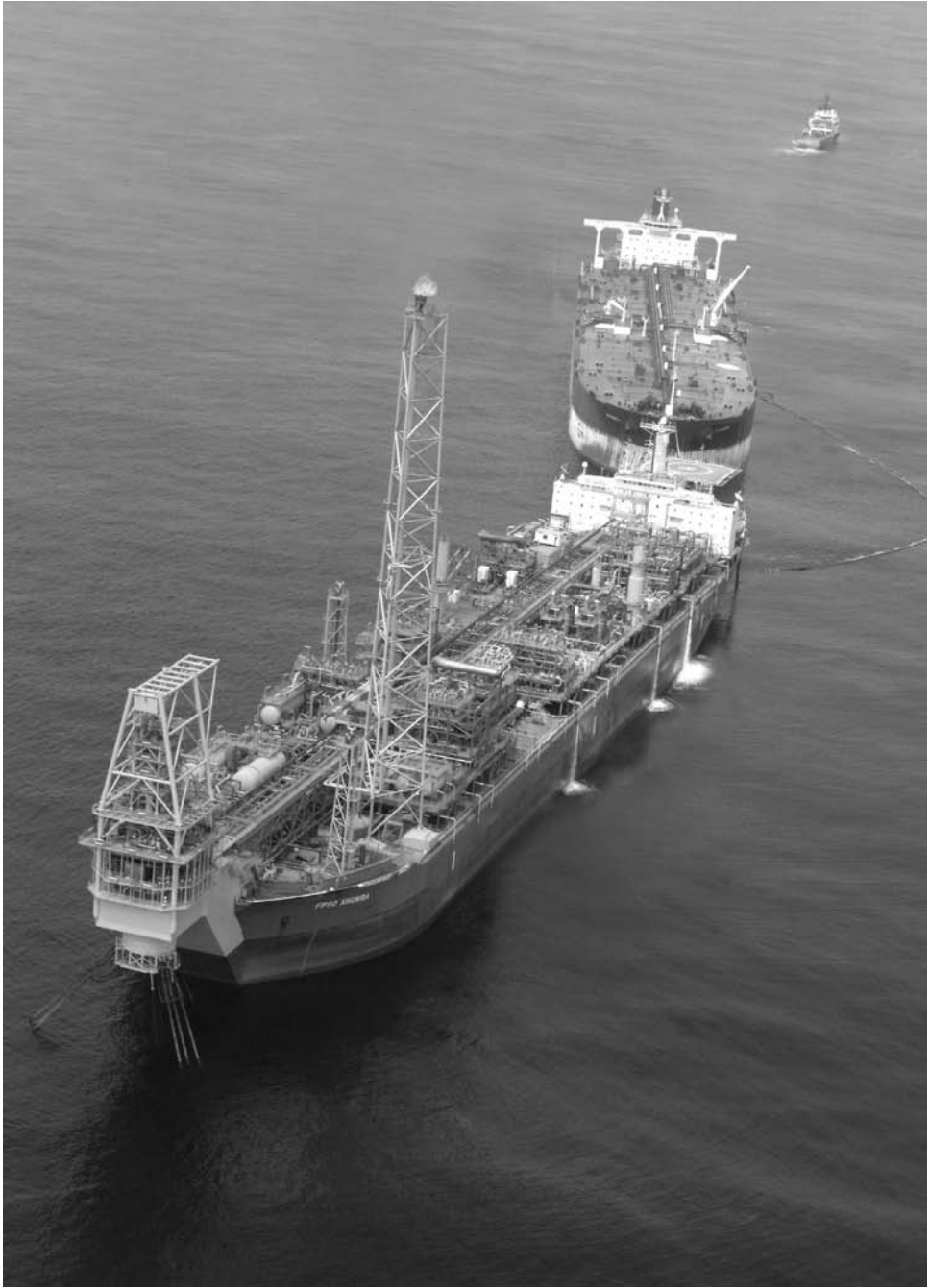
Figure 1.5. (cont.) (c) A photograph of a modern FPSO with an external turret mooring in a tandem export arrangement (courtesy of SBM Offshore NV).
