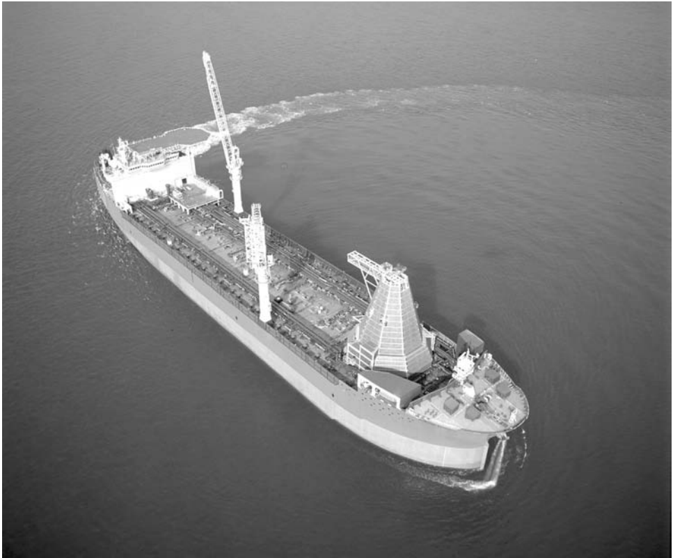
Figure 9.17. (cont.) (b) A photograph of an FPSO with an internal turret-mooring system (courtesy of Samsung Heavy Industries).
