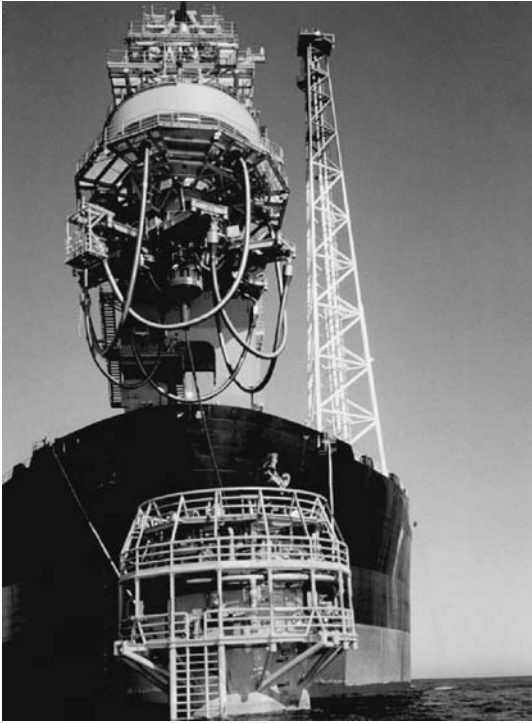
Figure 9.18. A photograph showing the installation of an external disconnectable turret during the connection operation (courtesy of SBM Offshore NV).
