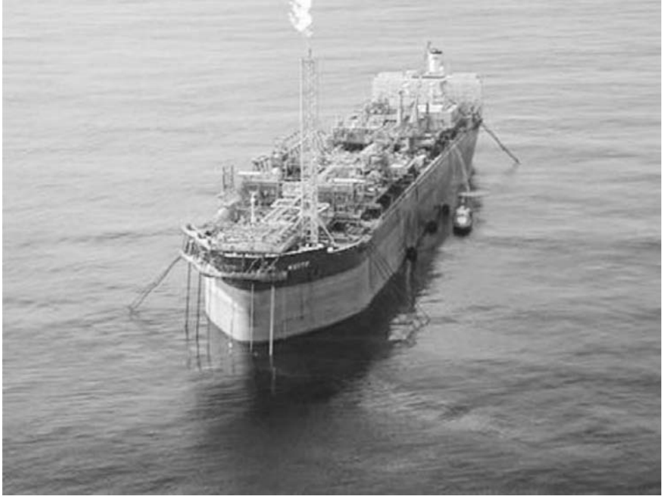
Figure 9.9. A spread-moored FPSO (courtesy of Samsung Heavy Industries).
