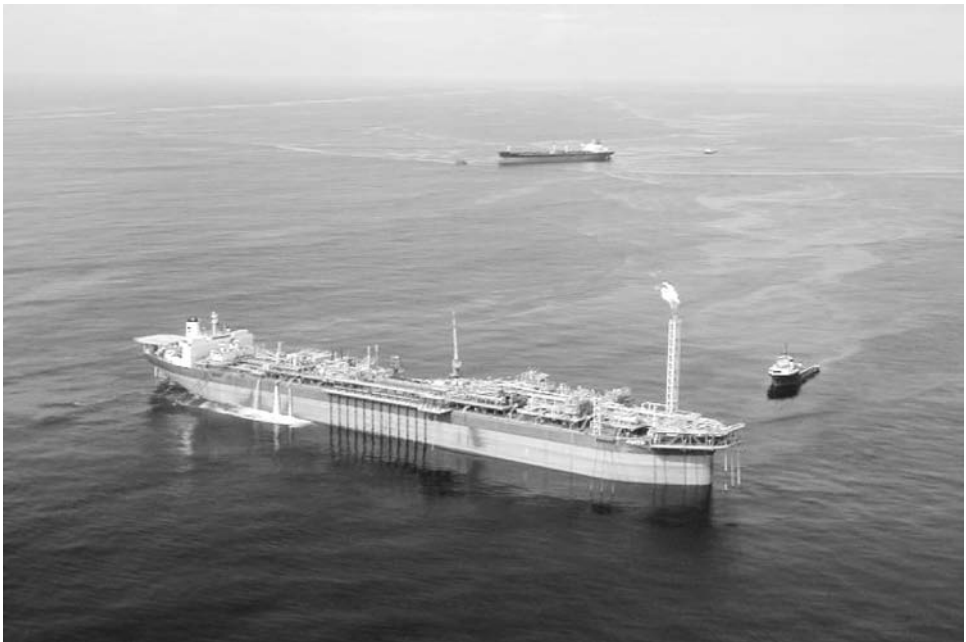
Figure 9.22. A photograph of an export arrangement with a CALM buoy-moored shuttle tanker located at a distance from an FPSO (Adhia et al. 2004; courtesy of American Society of Mechanical Engineers).
