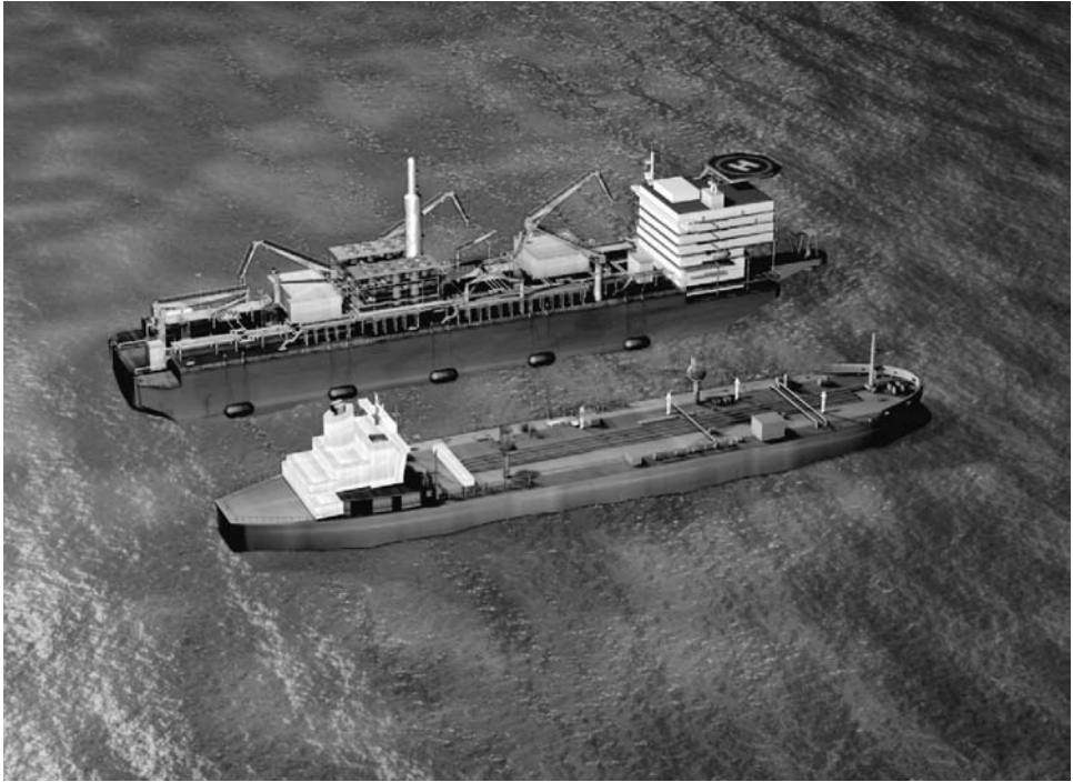
Figure 9.21. A computer graphic of a side-by-side export arrangement for an FPSO (Adhia et al. 2004; courtesy of American Society of Mechanical Engineers).
