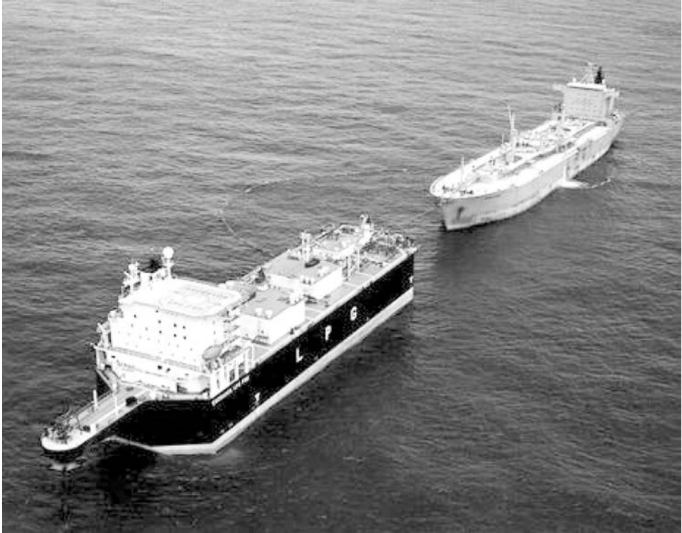
Figure 9.20. A photograph of a tandem export from an LPG FPSO (Adhia et al. 2004; courtesy of American Society of Mechanical Engineers).
