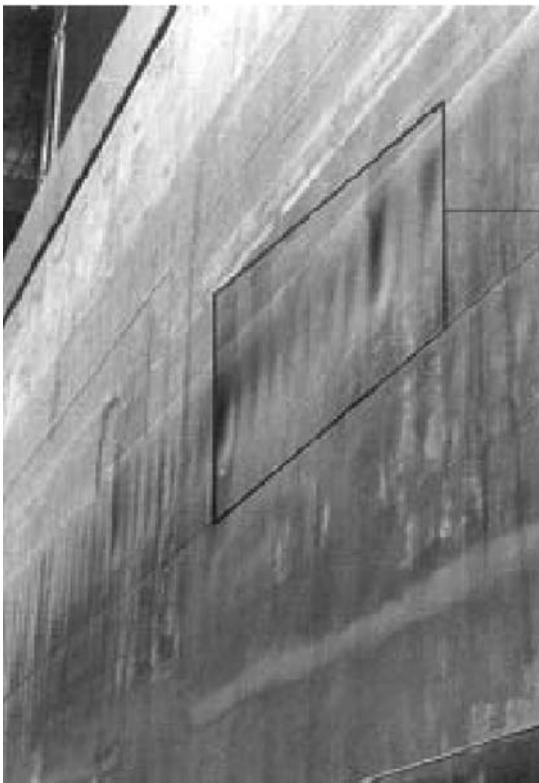
Figure 4.4. Plastic deformation on side shell structure of a trading ship due to ice loads (Kujala 1994).
