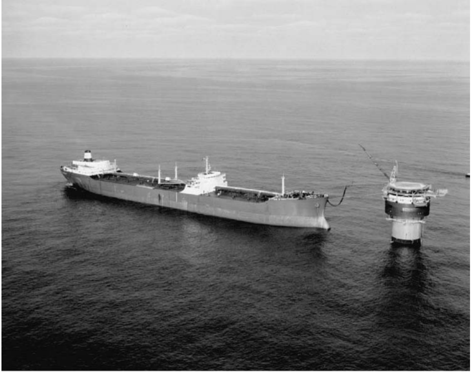
Figure 9.14. A vessel moored at a SPAR (courtesy of SBM Offshore NV).
