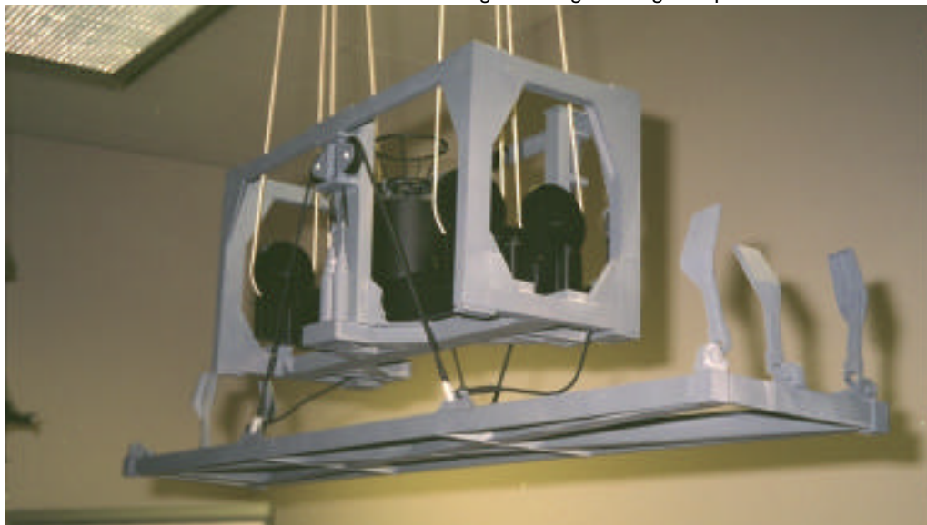
FIGURE 25. 1/16th scale model of the August Design Intelligent Spreader Bar
