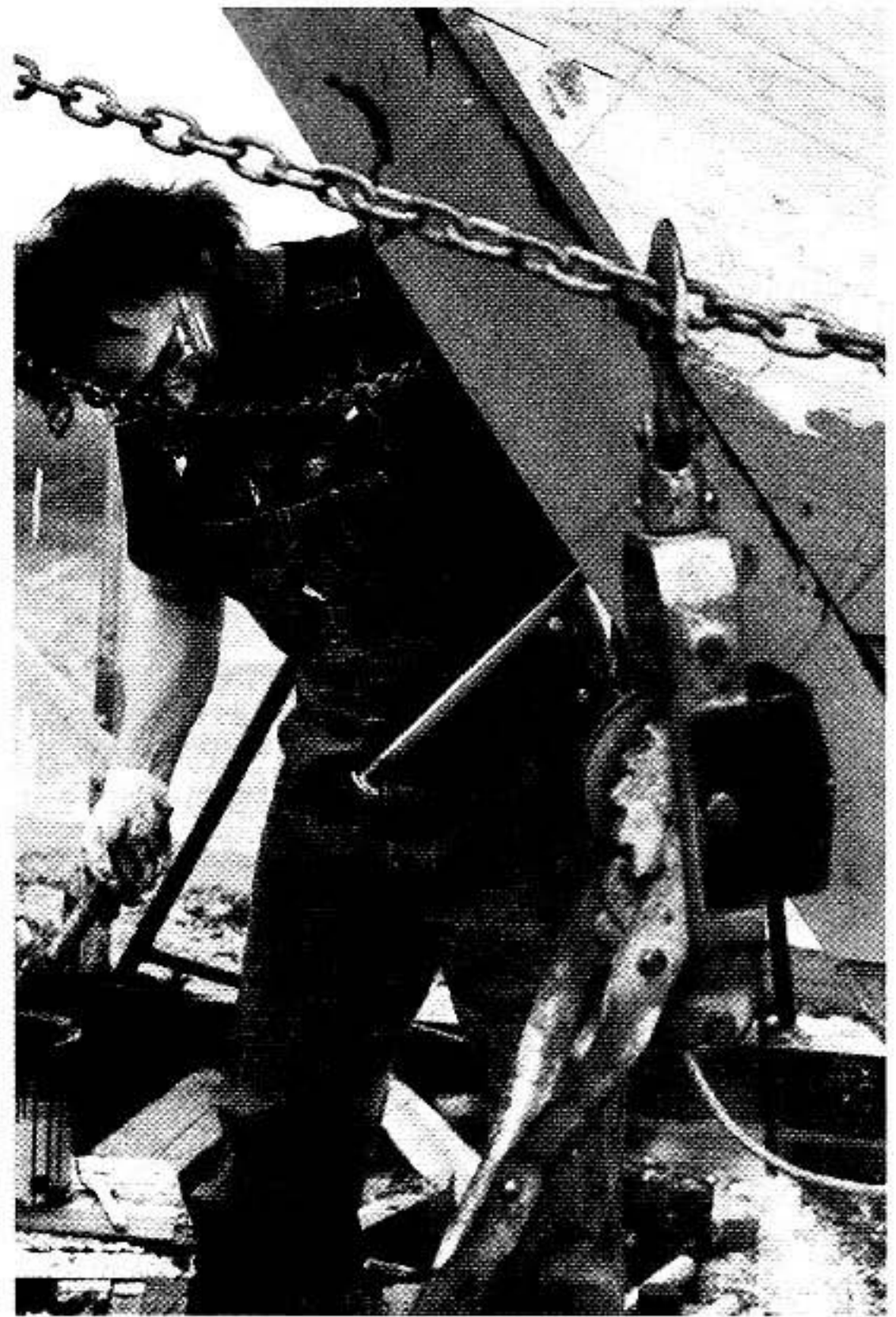
Driving in a drift bolt to fasten deadwood and sternpost. The timbers are sealed with red lead. (Courtesy Kortchmar & Willner)
