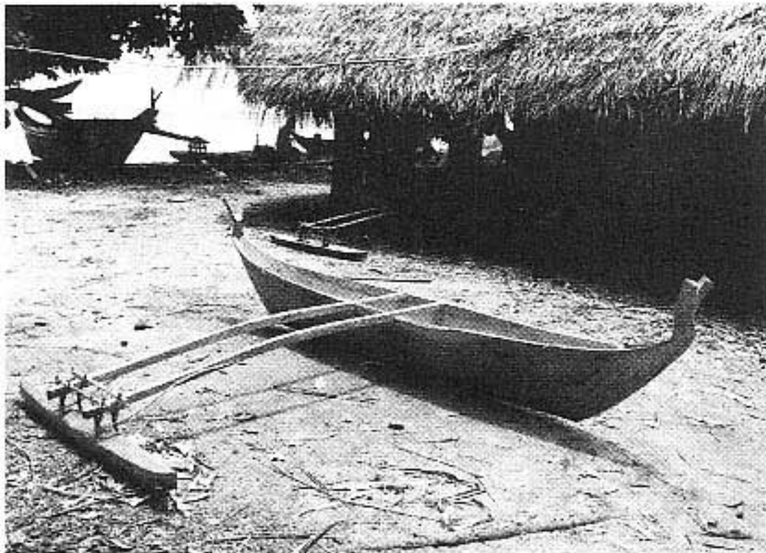
The Polynesian outrigger log canoe finished, before paint or rig. If you look closely at the bow, you can make out the two lashings that hold this separate piece in place. (Courtesy Stephen J. Winter)
