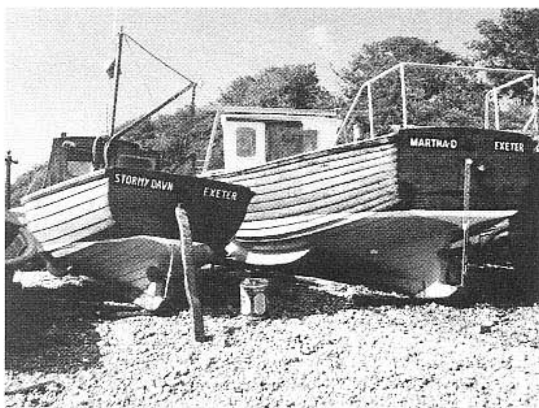
Lapstrake fishing vessels on the beach in Kittery, Maine. (Courtesy Alan Salisch)
