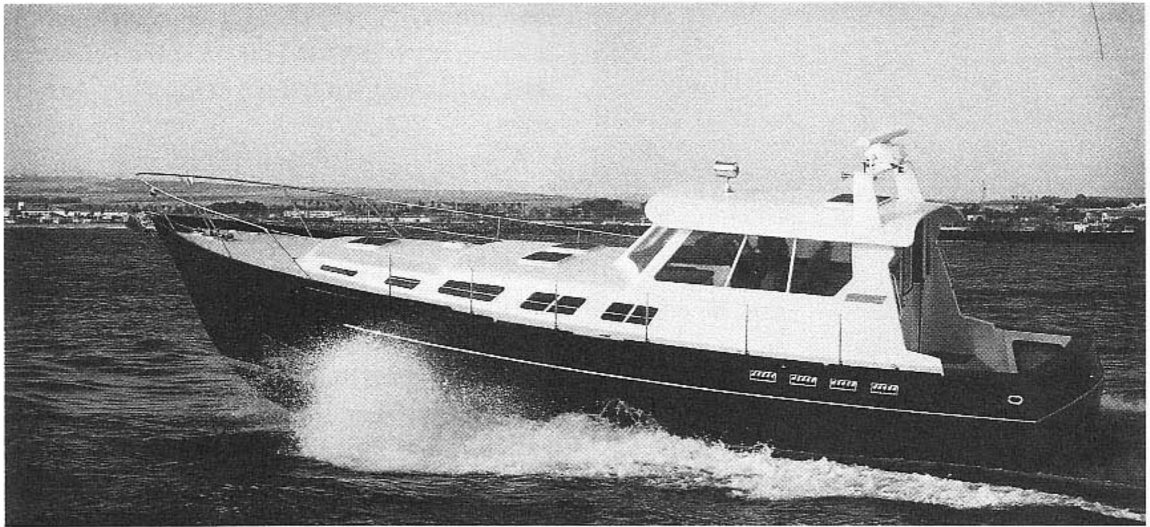
The Westbourne-44 high-speed Express Cruiser designed by the author. Constructed entirely of Baltek DuraKore and balsa-core panels, this boat came in under its predicted weight and has a top speed of 36 knots. (Courtesy Bob Grieser)
