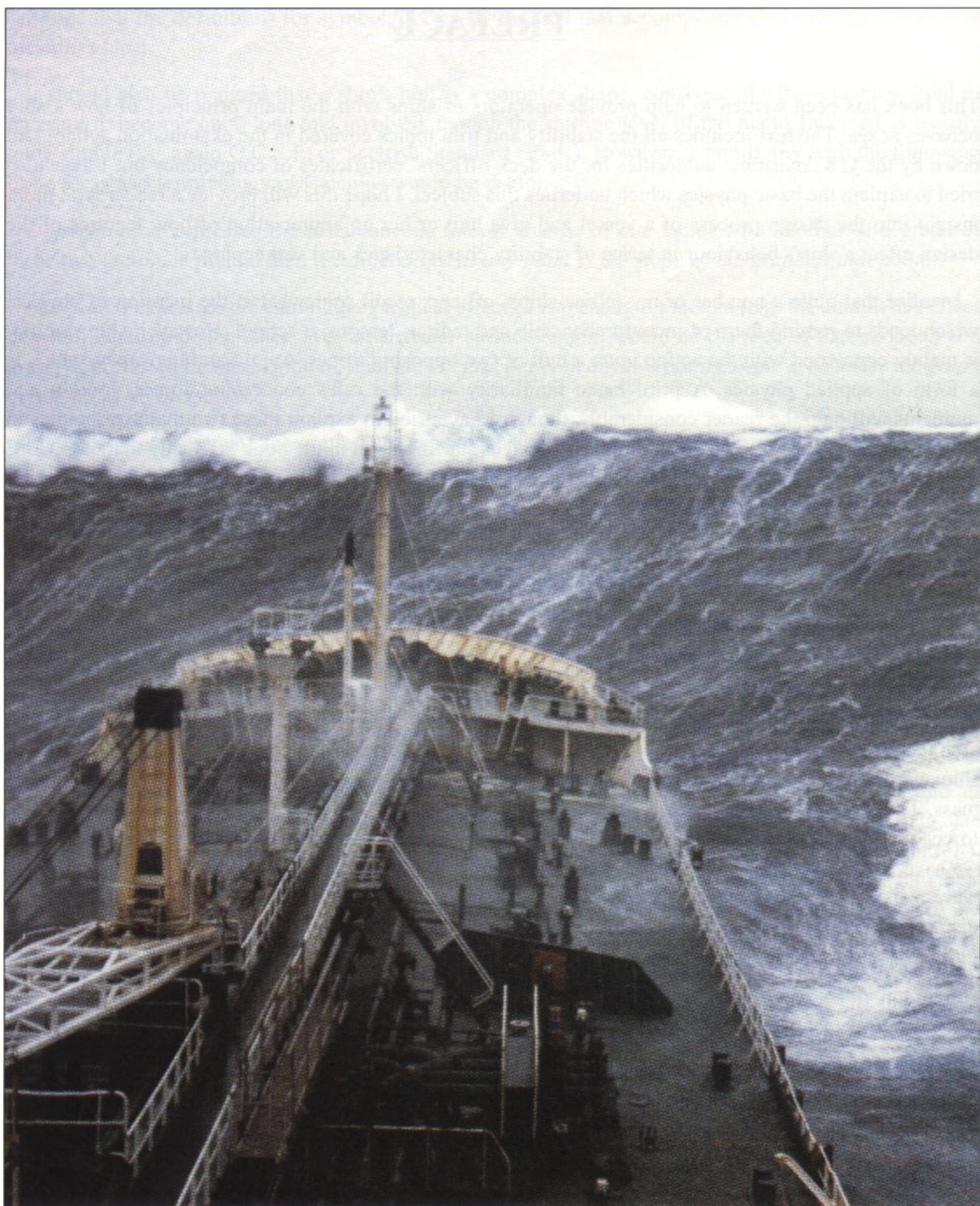
Heavy weather is a test of the ship's state of loading in terms of both stability and strength.
