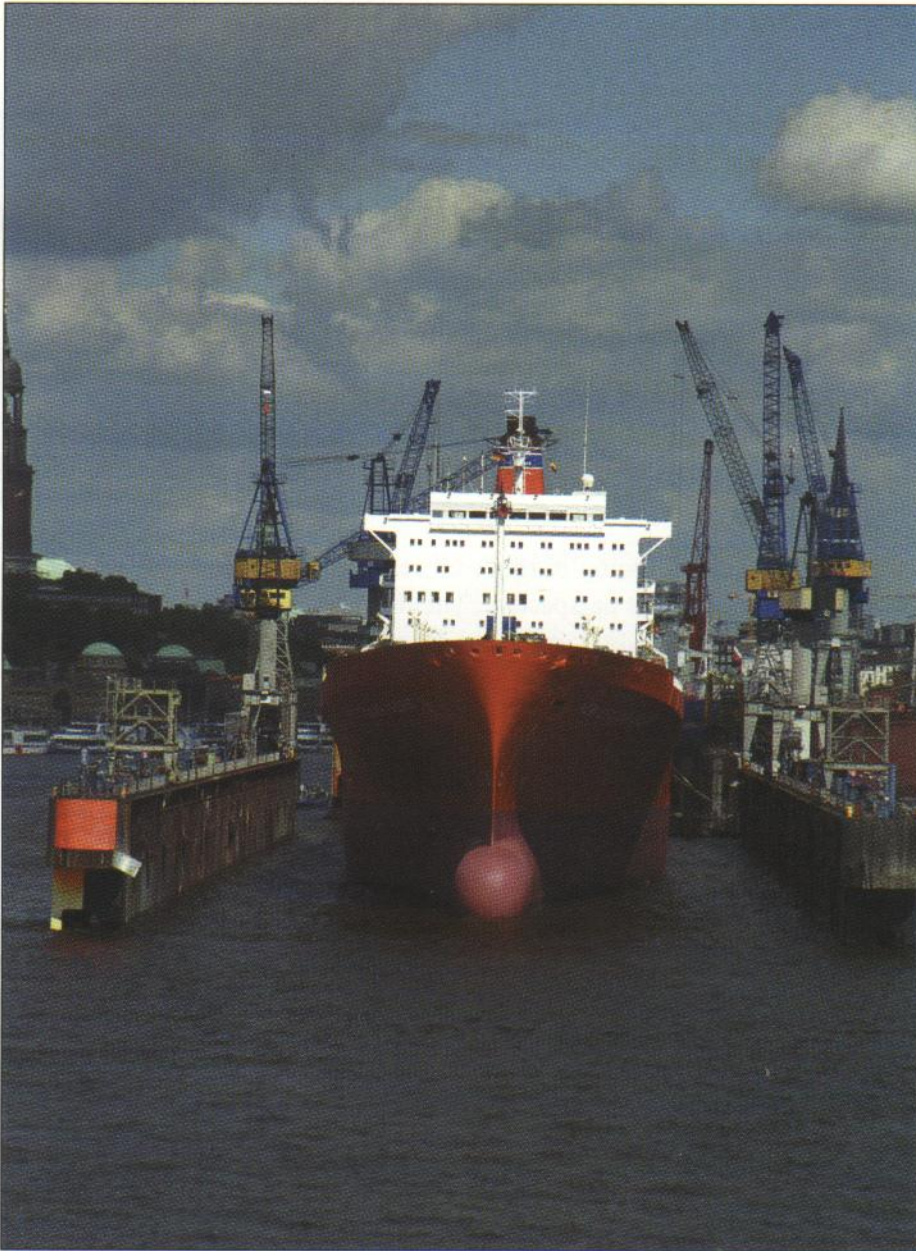
MV New Zealand Pacific at Blohm & Voss ag floating dock Hamburg. During the docking process, careful attention is needed to ship stability. (See chapter 6)
